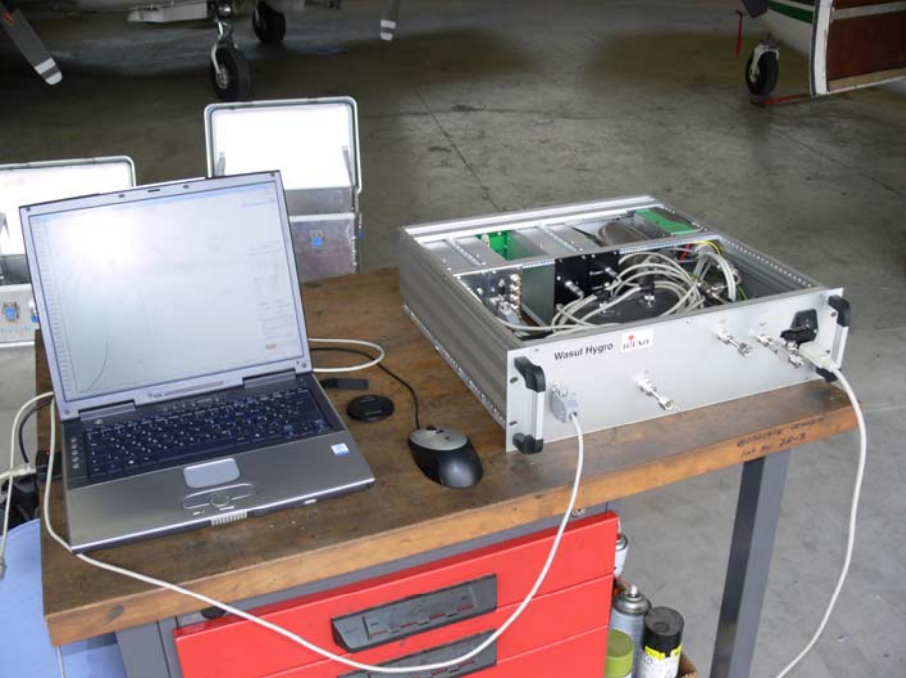
Figure 2. The WaSul-Hygro instrument before installation on the aircraft.
